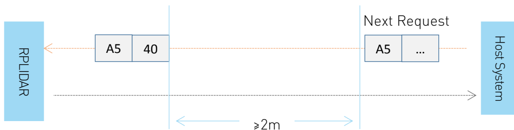
Figure 4-3 The Timing Sequence of a RESET Request
