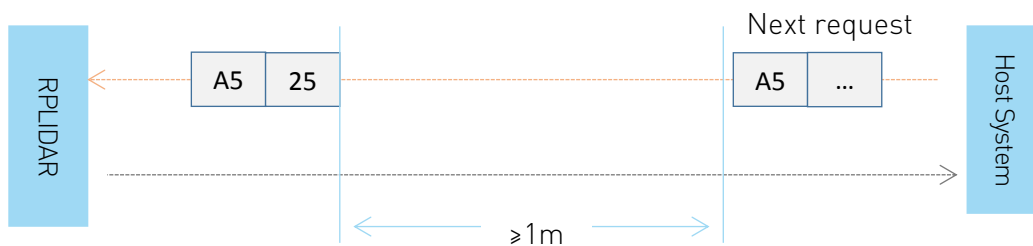
Figure 4-2 The Timing Sequence of a STOP Request
