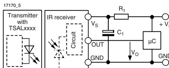
$R_1$  and  $C_1$  are recommended for protection against EOS. Components should be in the range of  $33 \text{ k}\Omega < R_1 < 1 \text{ k}\Omega$ ,  $C_1 > 0.1 \text{ }\mu\text{F}$ .
