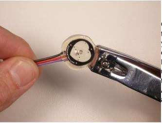
Once the hot glue has cooled (wait for it!) the blue tape will peel off very easily. Check your work to make sure that there are not exposed electrical connections!
