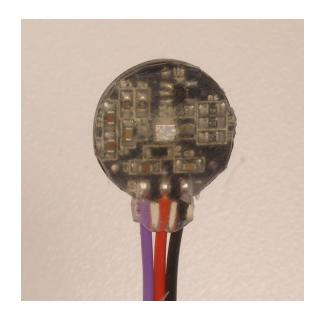
This is the basic Pulse Sensor Hot Glue Seal, It's also got the clear vinyl sticker on the front face. We're calling this 'Water Resistant', ready to be handled and passed around from fingers to earlobes or whatever. It is not advised to submerge or soak the Pulse Sensor with this basic seal.
