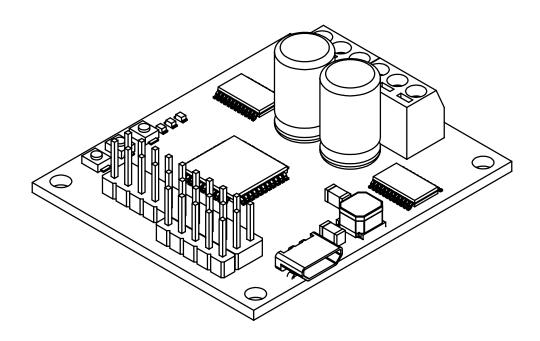
RoboClaw 2x7A, 34VDC Dual Channel Brushed DC Motor Controller
