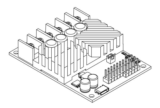
RoboClaw 2x15A, 34VDC Dual Channel Brushed DC Motor Controller
