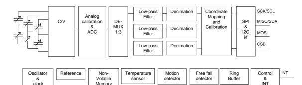
Figure 1. SCA3000 Block Diagram.
