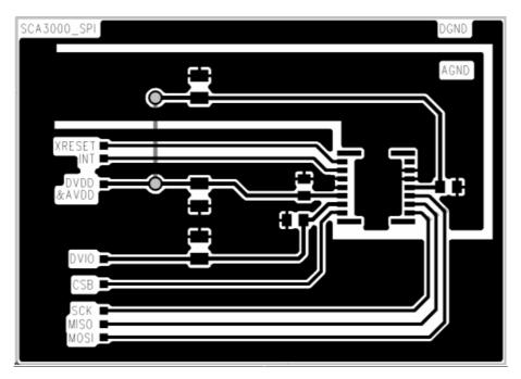
Figure 18. Recommended PWB layout for SCA3000 with SPI interface (not actual size, for reference only).
