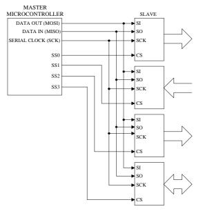
Figure 5. Typical SPI connection.
