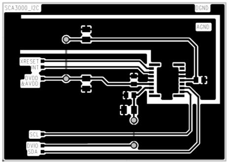
Figure 19. Recommended PWB layout for SCA3000 with  $l^2C$  interface (not actual size, for reference only).
