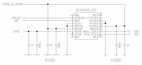
Figure 16. Recommended circuit diagram for the SCA3000 with I<sup>2</sup>C interface.
