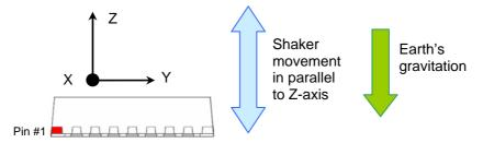
Figure 24. SCA3000 movement in Z-axis bandwidth measurement.
