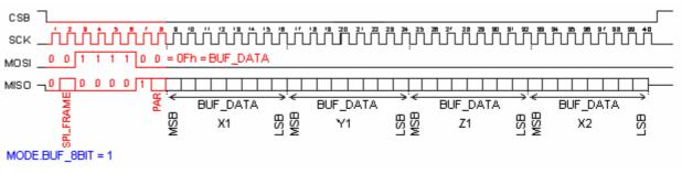
Figure 9. An example of output ring buffer read operation.
