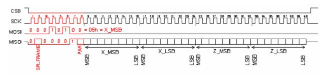
Figure 8. An example of decremented read operation.
