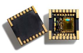
SCA3000 Series 3-axis accelerometer
