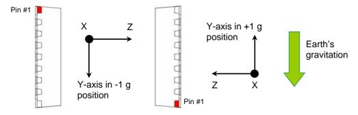
Figure 21. SCA3000 positions for Y-axis sensitivity measurement.
