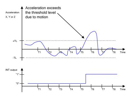
Figure 3. Motion detector operation.
