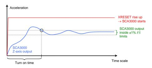
Figure 25. Turn-on time definition for one axis.
