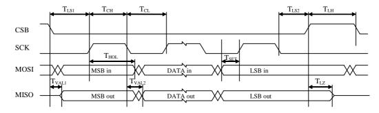
Figure 11. Timing diagram for SPI communication.
