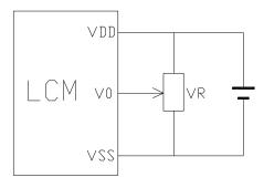
V<sub>DD</sub>~V₀: LCD Driving voltage
