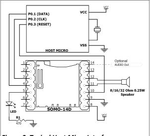
Figure 3: Typical Host Micro Interface
